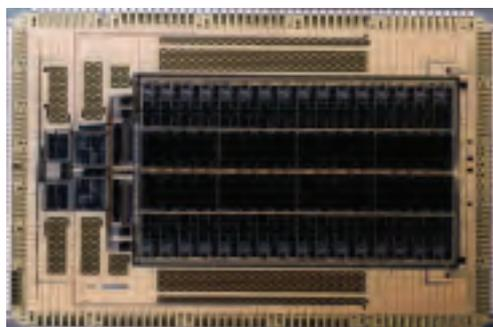
**Ultra-low power digital filtering chip for DSL.
