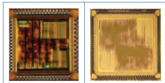
**BLAST Chips, 19Mb/s and 28.8Mb/s 4x4 MIMO - HSDPA, Bell Labs Australia, 2002 & 2003**
